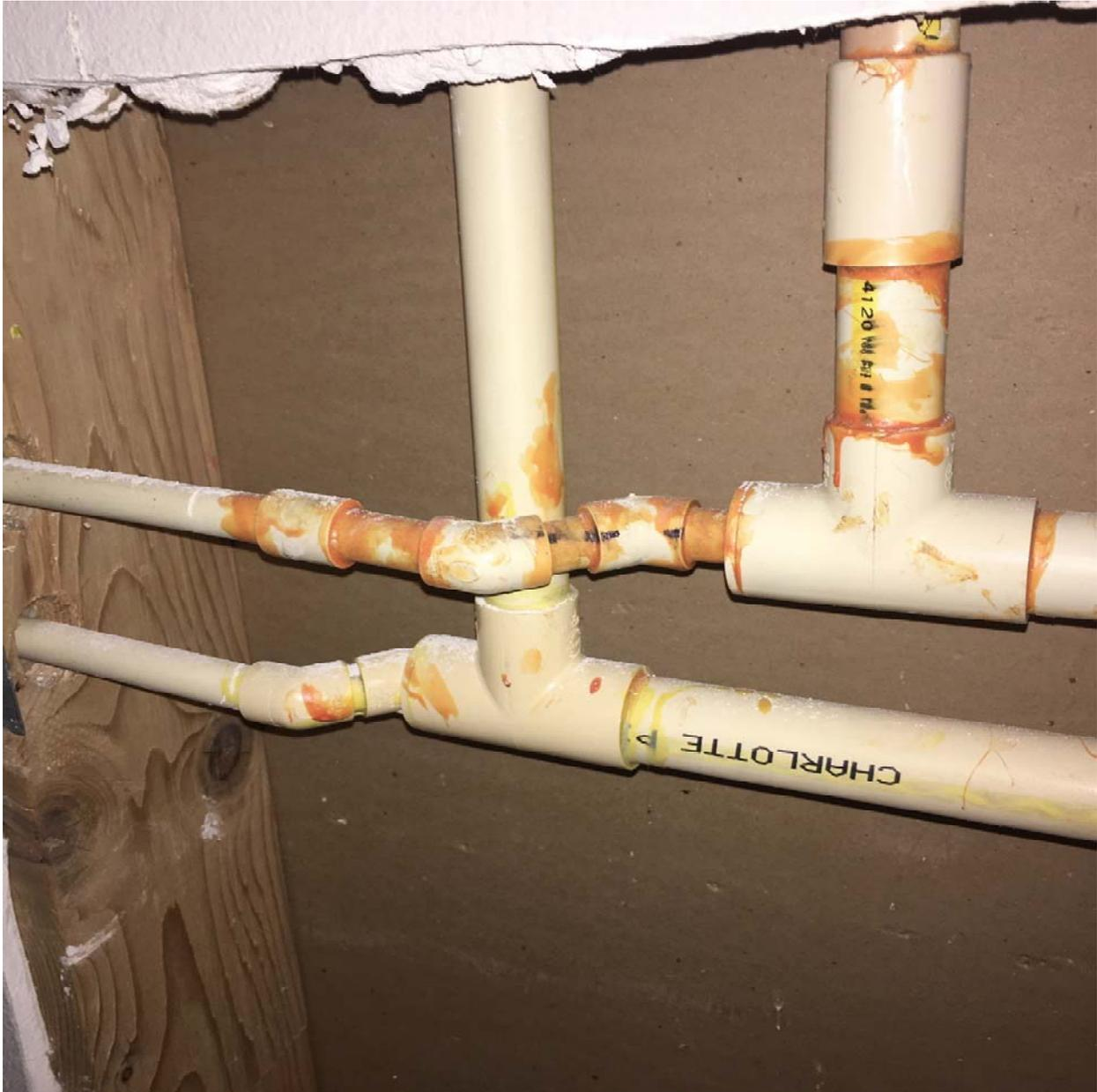
57. The following photos are of the failed fittings from Baker's second FlowGuard Gold leak and the area of the leak:
